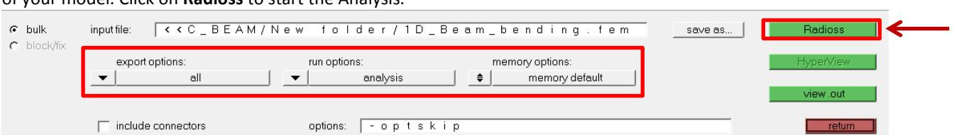
4. A new solver window will open. Once you see ANALYSIS COMPLETED close the solver window.
