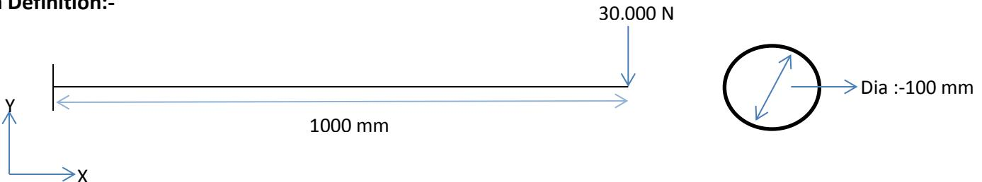
A 1000mm in length, a solid circular Beam of 100mm diameter is subjected to a bending load of 30000 N in Y-direction and it is fixed at the other end the deflection and stress values has been calculated using the below method. Then the same problem is solved in HyperMesh and then showing the comparison to both the results that is values of deflection and stress with hand calculation and values of deflection and stress by using the software.
