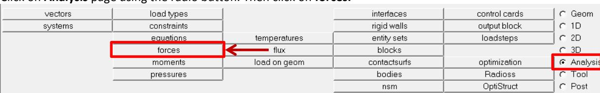
5. Click on the **nodes** and select the node as shown. Make sure the toggle is set to **global system**, Enter **-30000** in **magnitude =**, and select **y-axis** as the direction of force. Keep all the other parameters as shown in the image. Click **create**.
