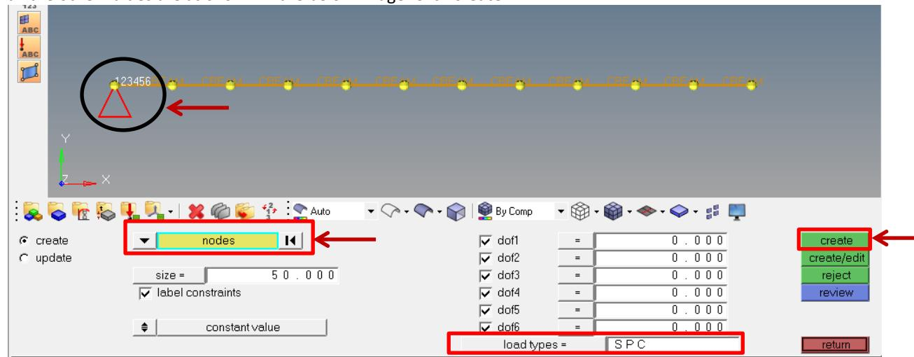
*dof 1, dof 2 and dof3 means translation along x-axis, y-axis and z-axis. And dof 4, dof 5 and dof 6 means rotation about x-axis, y-axis and z-axis respectively. If any dof is checked that means it is fixed and if any dof is unchecked that means that the component is free to translate or rotate in that particular dof.*
